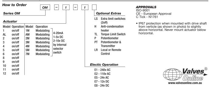
E11 - 415v AC Ordering Example: OM-1-1 240 VAC Electric Actuator c/w lever (spanner face shaft) manual override, 90° turn on/off
